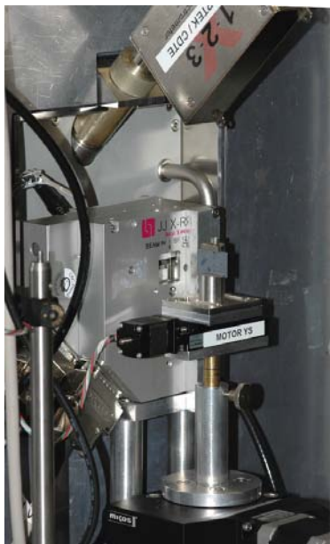
Figure 5.2: Photo of the setup sketched in figure 5.1. The spectrum of the plasma radiation can be constantly monitored with an Amptek Si-drift detector mounted above the sample.
