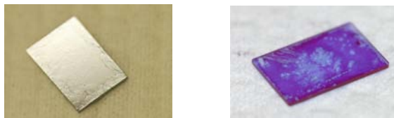
Figure 2.5: Photos of the samples used in the time resolved diffraction experiments using pulsed laser excitation. Left: Unlabeled DOPC multilayers on polished Si wafers. Right: Texas-red labeled DOPC multilayers at a Texas-red-DHPE mole fraction (%TR) of 5.
