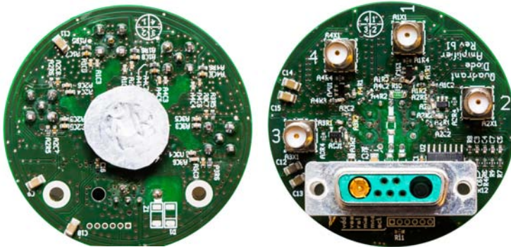
Figure 3.4: Photos of the printed circuit board (PCB) of the high bandwidth preamplifier. Left: Front view. The quadrant APD is located in the center of the PCB. It is covered by a approximately 30\mu\text{m} thin Al-foil in order to prevent an exposure to ambient light, dust contamination and humidity uptake. Right: Back view. Amplified signals are routed to four SMA connectors. Communication with the on-board micro controller, high voltage biasing of the APD and supply voltages are provided via a Conec mixed Sub-D connector.
