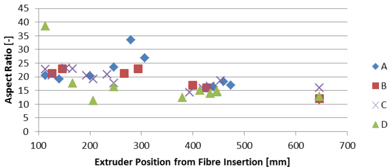
Figure 7: Fibre aspect ratio along the different extruders at 30% Wf and 200 rpm
