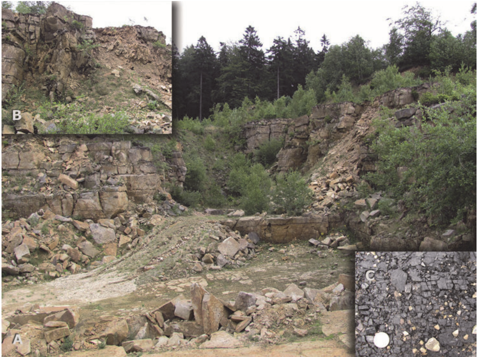
Fig. 4 The coal coulee in the southern part of the Obernkirchen sandstone quarries. (A) showing the fault area with its heavy shear fracturing of the sandstone banks (B) and a natural surface outcrop of the ‘German Wealden’ coal (C) . Unfaulted, the coal seam layer would have had to be mined some 2–4 m below. Scale in (C) : 1 € coin.
