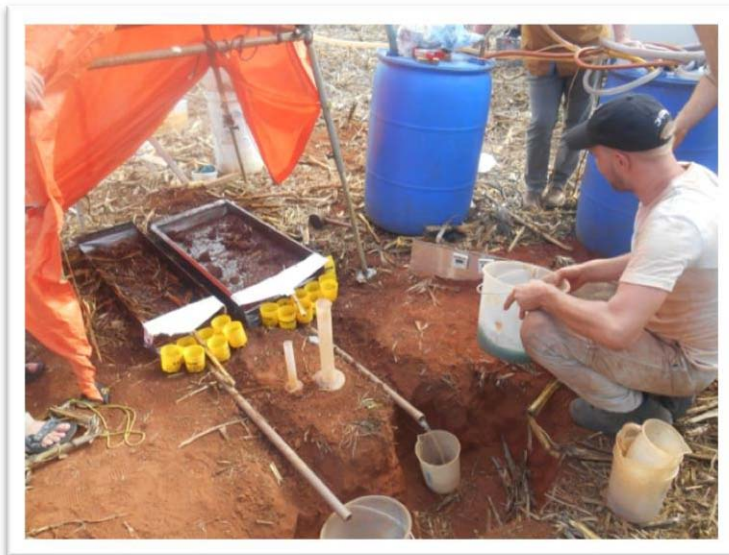
Measuring soil erosion under controlled conditions
