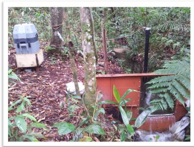
Microcatchment weir in Campo Verde, Mato Grosso
